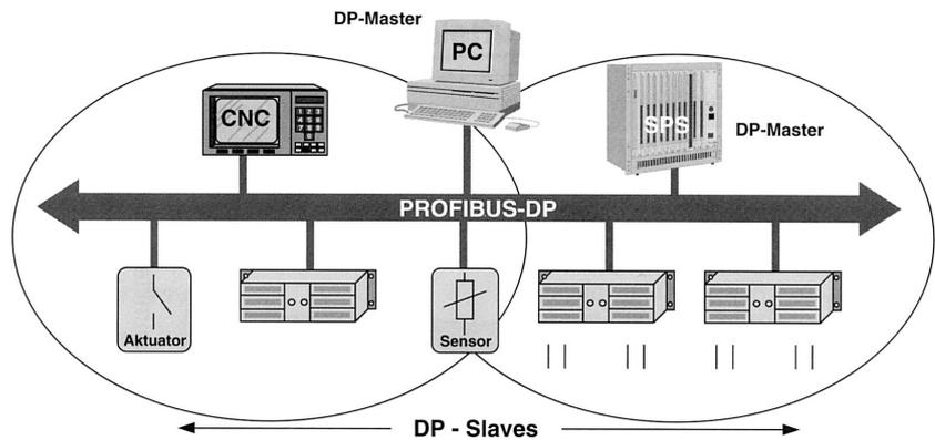
The PROFIBUS-DP network has a tree structure and the main branches are represented by the units and/or sub-networks managed by other Masters. In order to identify a unit of the network, users can assign a "DA" address to each unit which is communicated to the Master during it's initialization.
