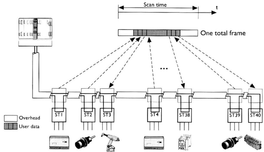
In this way a very high efficiency is obtained because the part of the message which doesn't contain information but only data for transmission control is reduced to the minimum. A network can connect up to 512 devices on a max. length of 400 mt. or up to 13 km by using a signal repeater. The typical transmission rate (baudrate) is 500 Kbit/s.
