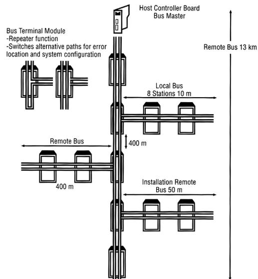
InterBus-S devices are distinguished in 4 different profiles, from 1 to 4. The differences are the length of transmitted data (1 and 2) and the possibility both to receive and to transmit data (3 and 4). Profibus for example distinguishes only between programmable and not programmable devices (class 2 and 1).
