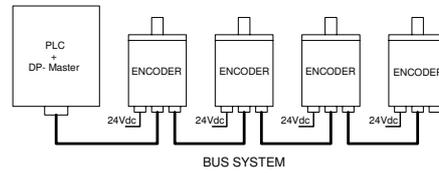
The Master can connect up to 125 Slaves, divided into groups of 32, through a special two wire cable designed for high speed transmission up to 12 Mbits.
