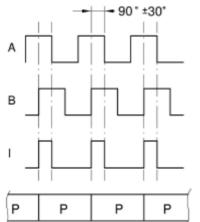
As the sensor is moved along the magnetic tape, it detects the displacement and produces an output signal equivalent to that of an incremental encoder or a linear scale. The signal output is proportional to the measuring speed and to the displacement of the sensor. Resolution after quadrature (4 edge reading) can be determined by the ordering code on the sensor.
