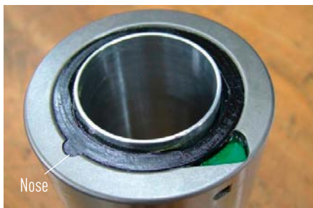
Fig. 4.4 Before assembly ensure that wipers are seated correctly
