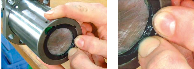
Fig. 4.7 Fixing the wiper while slowly screwing nut onto shaft
