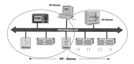
The PROFIBUS-DP network has a tree structure and the main branches are represented by the units and/or sub-networks managed by other Masters.
