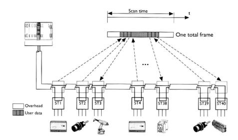
In this way a very high efficiency is obtained because the part of the message which doesn't contain information but only data for transmission control is reduced to the minimum.
