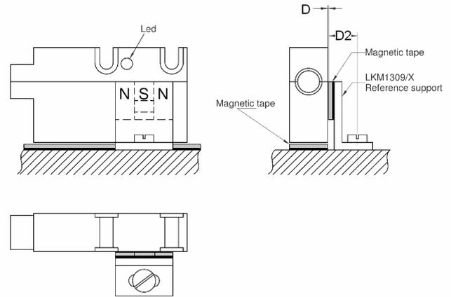
**D:** gap to be kept between sensor and LKM1309.
