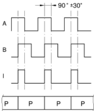
As the sensor is moved along the magnetic tape, it detects the displacement and produces an output signal equivalent to that of an incremental encoder or a linear scale. The signal output is proportional to the measuring speed and to the displacement of the sensor. Resolution after quadrature (4 edge reading) can be determined by the ordering code on the sensor.
