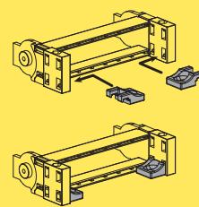
Reducers mounted on the outer radius
