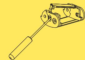
Special tool to remove the connecting pivots:
