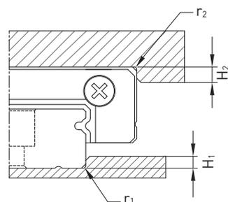
Fig. 4.25 Shoulder heights and fillets – MG and PM series
