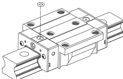
Alternatively, lubrication of the block can also be carried out from above. In doing so, an O-ring is used as a seal. The size of the O-ring is to be found in Table 6.4. The O-ring is not included in the standard shipment.
