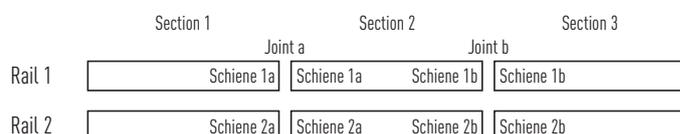
Fig. 4.28 Identification of jointed multi-part rails\*
