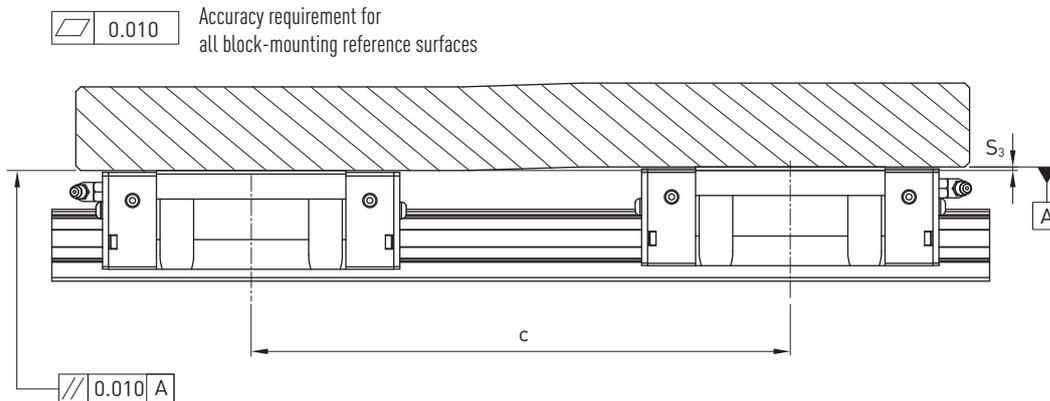
Fig. 4.21 Maximum height tolerance  $S_3$
