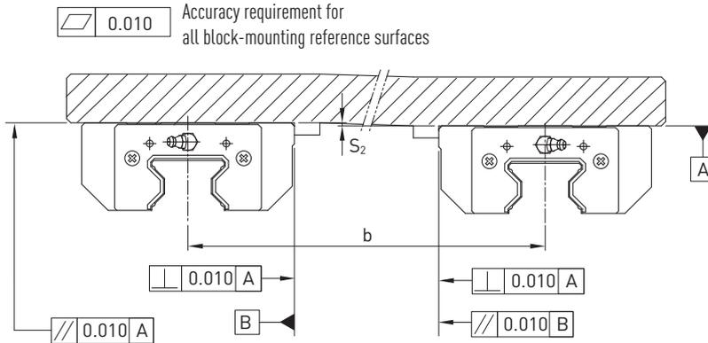
Fig. 4.20 Maximum height tolerance  $S_2$
