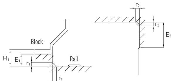
Fig. 4.26 Shoulder heights and fillets – RG/QR series
