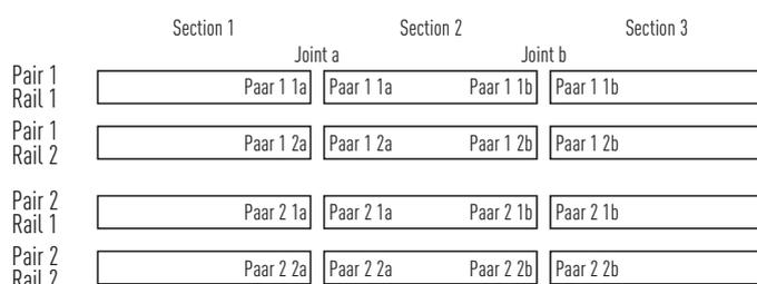
Fig. 4.29 Identification of jointed multi-part paired rails\*
