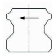
Fig. 4.2 Identification of the datum plane of a short rail
