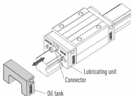
Lubrication passes from the oil cartridge via the connector to the lubricator which then lubricates the track of the rail. Due to the specific design of the oil tank, the block can be assembled in any position without influencing the lubrication effect. The replacement intervals of the oil tank depend heavily on the loads and the environmental conditions. Environmental influences such as high loads, vibrations and dirt shorten the replacement intervals.
