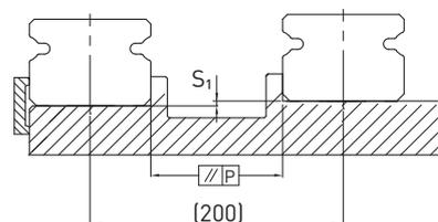
Fig. 4.18 Parallelism of the reference surface P – PM series
