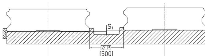
Fig. 4.16 Parallelism of the reference surface P – WE series
