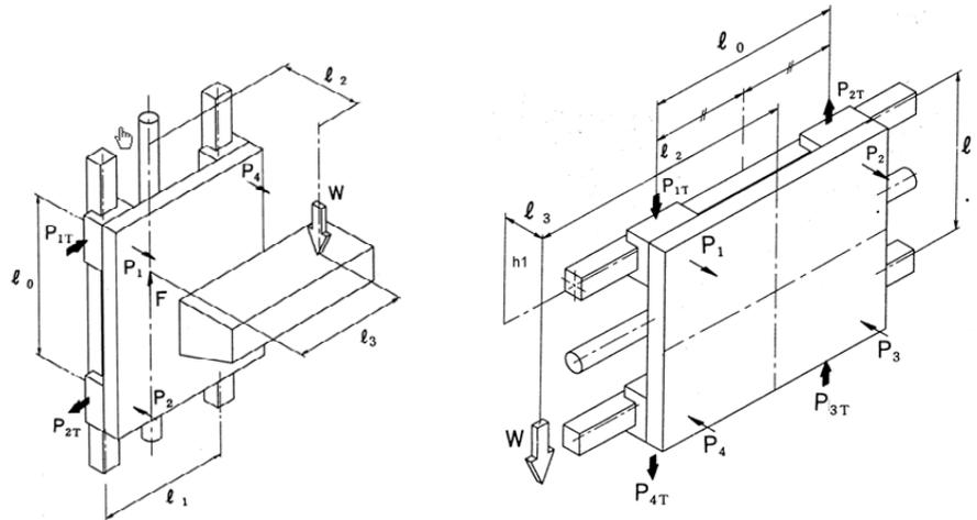
Fig. 6.18 Mounting positions of profile rails
