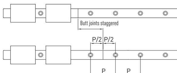
Fig. 4.30 Configuration of jointed multi-part rails
