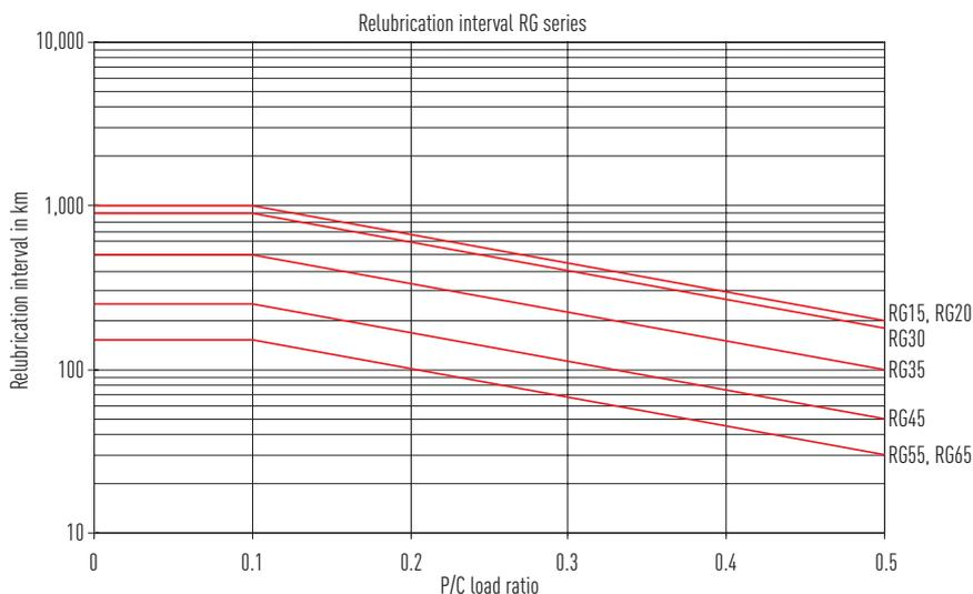
Fig. 6.31 Load-dependent relubrication intervals for grease lubrication – RG series
