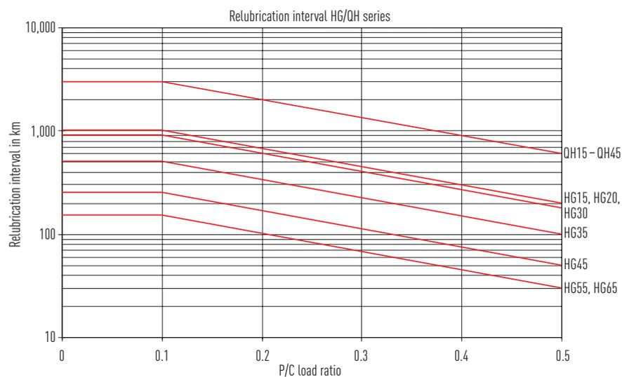
Fig. 6.26 Load-dependent relubrication intervals for grease lubrication – HG/QH series
