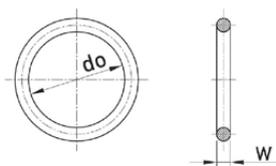
Fig. 6.15 O-ring to cover the lubrication connection on the top
